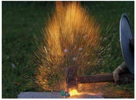
A li-ion battery cell exploding after being hit by a hammer
